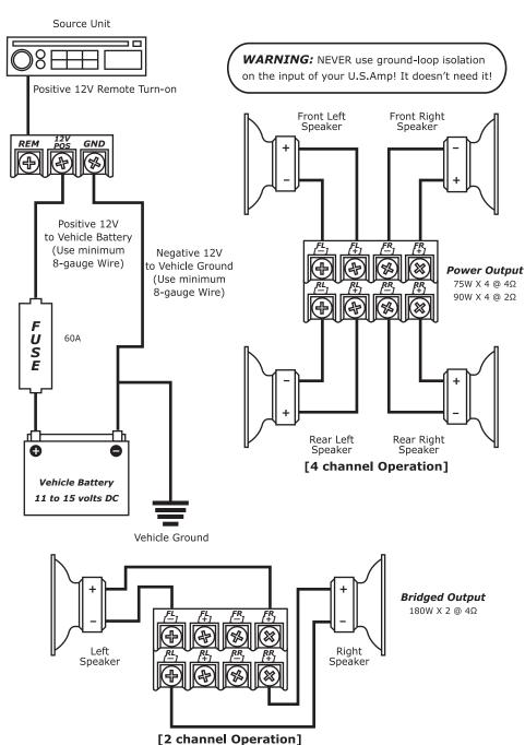
DO NOT OPERATE AX-4360C BRIDGED MONO AT LESS THAN  $4\Omega$  PER BRIDGED CHANNEL
